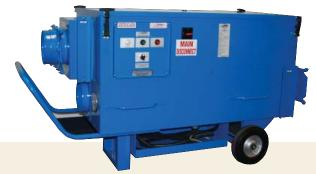
The DESICAIR<sup>®</sup>Series 1000 & 2000 models are industrial duty, dry desiccant dehumidifiers. Engineered to operate under severe operating conditions, the DESICAiR<sup>®</sup>Series 1000 & 2000 uses the most advanced desiccant technology available to remove moisture directly from the air. Humidity can be reduced to levels well below that which is achievable with a conventional refrigerant based dehumidification system.
